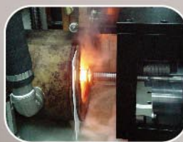
加熱淬火站及淬火液循環槽，設置線上回火裝製 Quenching and Tempering Station
