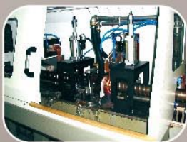
加熱淬火站及淬火液循環槽，設置線上回火裝製 Quenching and Tempering Station
